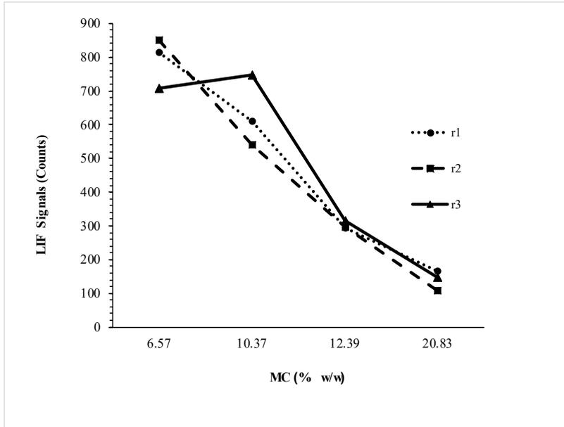
Figure 6. LIF signals in four MCs; in three replications ( $r_1, r_2, r_3$ ) LIF decreases with MC increasing. The rising LIF of MC 10.37 in third replication ( $r_3$ ) might be an outlier data.
