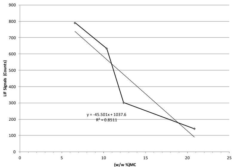
*Figure 7.* LIF variations with increasing MC; 85% of the moisture contents variations from 6.57% w/w increasing to 20.83% w/w can be explained by the linear model.
