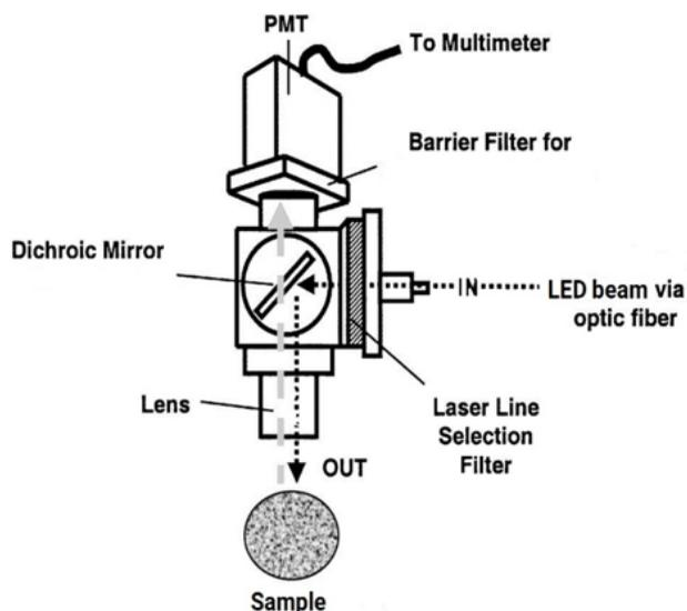
Figure 1. LIF Sensor; LED beam via optic fiber is directed to dichroic mirror. It enhances the beam and then reflects it 90° to the sample. Fluorescent API within sample is excited and emits fluorescent signal. Then, emitted light-induced fluorescence is collimated, filtered and converted to voltage and finally recorded to a computer.
