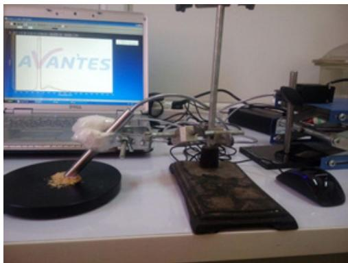
Figure 2. The LIF Test; Avalight-LED<sup>®</sup> compact produces pulsed or continuous spectral outputs, when a sample is excited at 405 nm, generating a specific emission peak at 492 nm.
