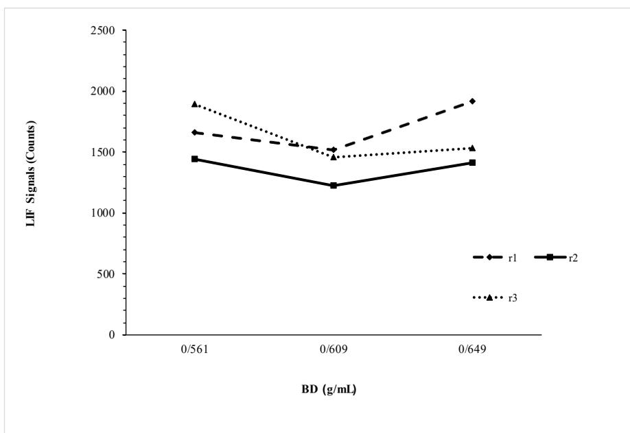
Figure 5. LIF signals in three bulk densities; the experiments was performed in three replications ( $r_1$ ,  $r_2$ ,  $r_3$ ) that LIF falling of BD 0.609 g/mL was the same for all.
