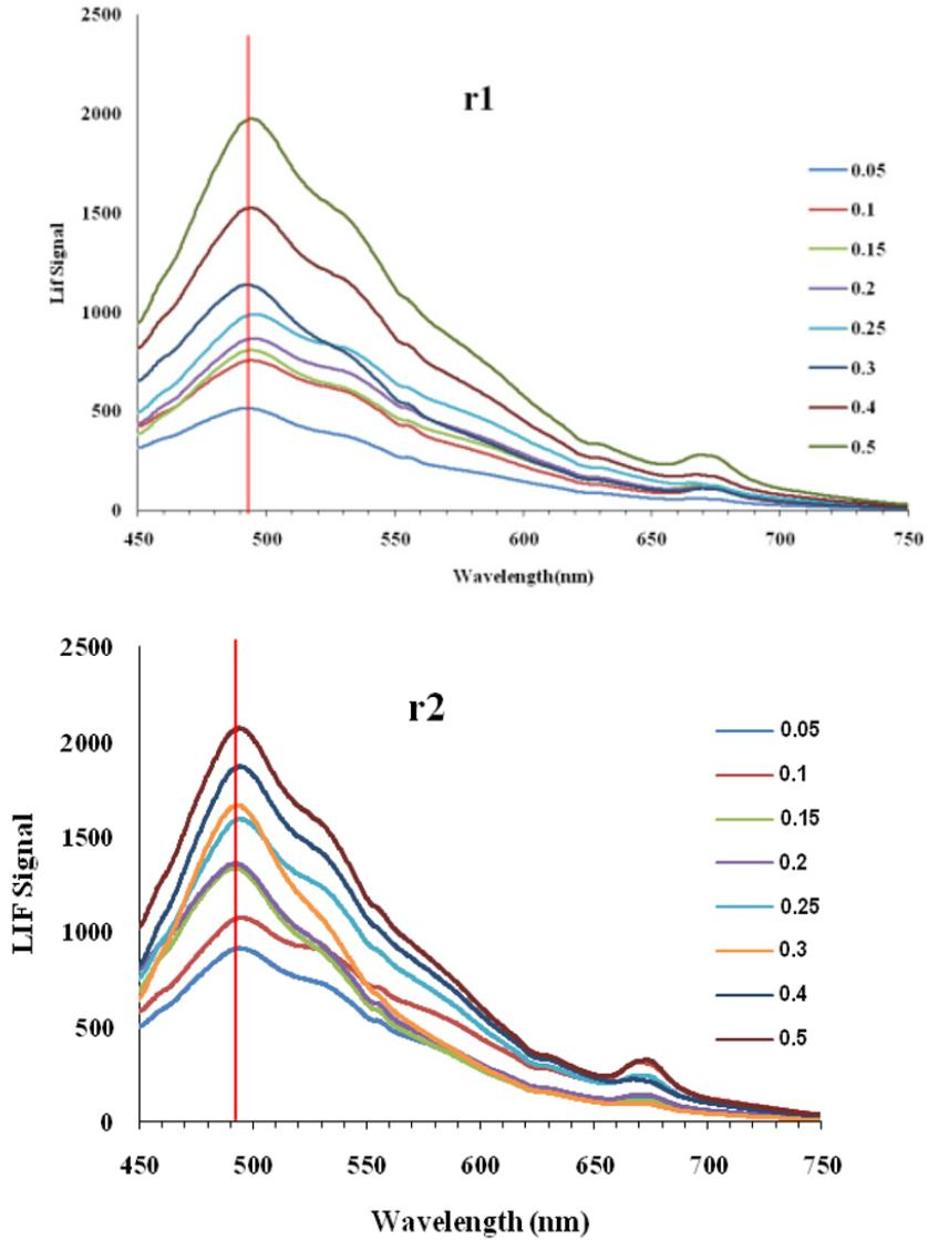
Figure 3. LIF peak was in 492 nm for all concentrations with 10% w/w moisture content and 0.65 g/mL bulk density in all three replications ( $r_1, r_2, r_3$ ).
