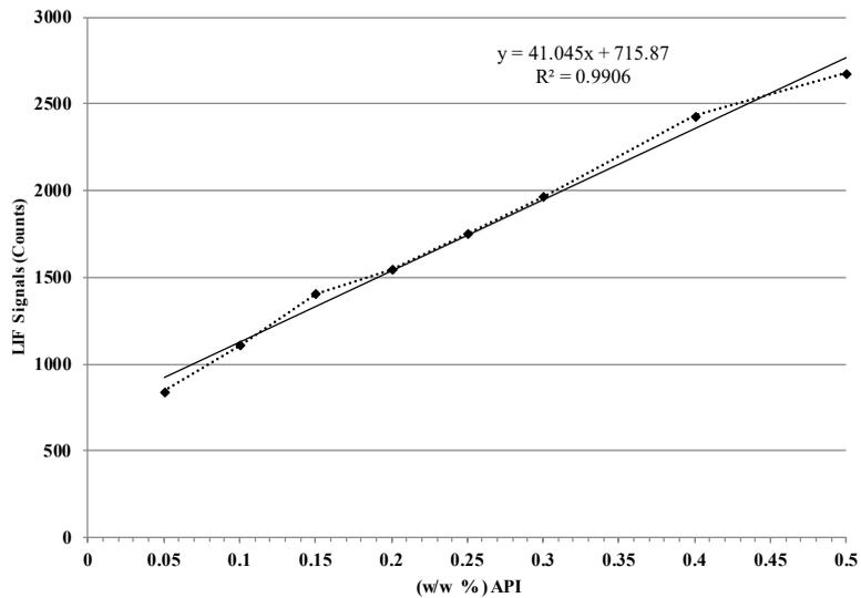
Figure 4. Linear variations in LIF with increasing API; increasing API caused a linear increase of fluorescence.
